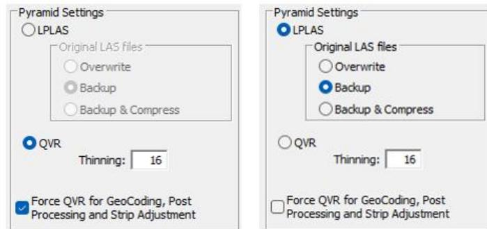
The LPLAS file format is compatible with any software able to read LAS and follows the ASPRS standards for the most up-to-date specifications for LAS. LPLAS files are useful for their improved pyramid performance and highly detailed point cloud display capabilities over the older QVR format. An example of this can be seen below.
