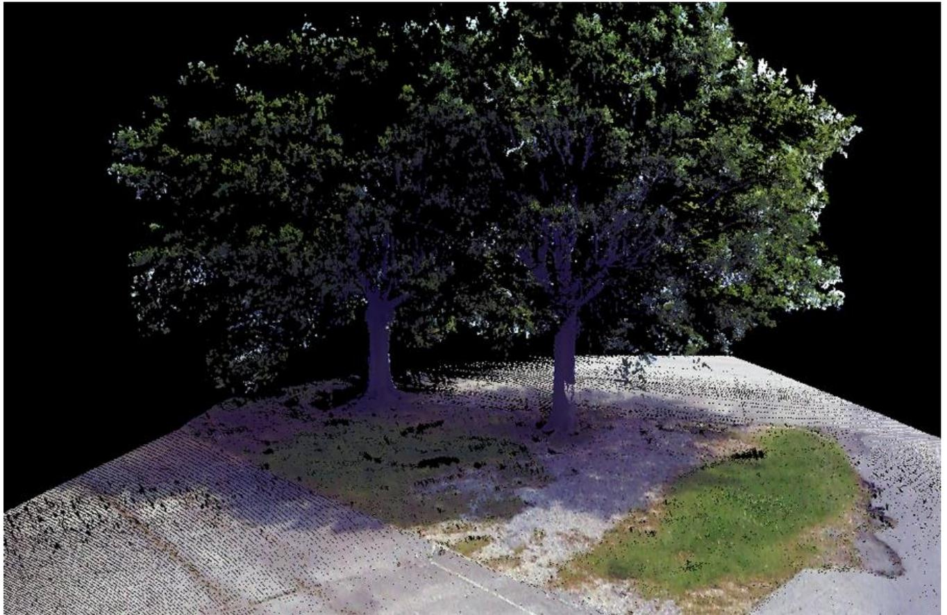
Figure 2 - Terrestrial LIDAR data displayed by RGB values
