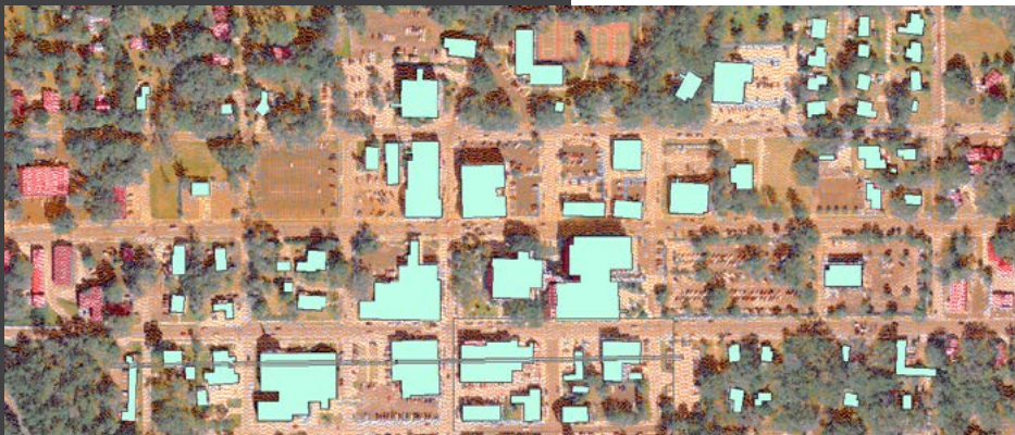
Figure 2 - View of classified and extracted buildings created using LP360's automatic building classification and extractor tool.
