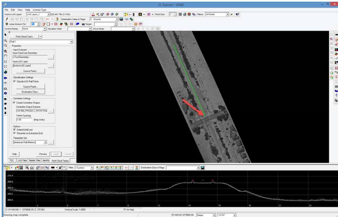
**Figure 3: Result of extraction a segment (Map View) and classified rail (Profile View)**
