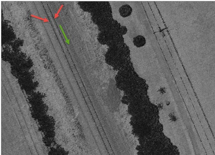
**Figure 2: "Seeding" the alignment (red arrows denote the rails, green the "seek" direction)**
