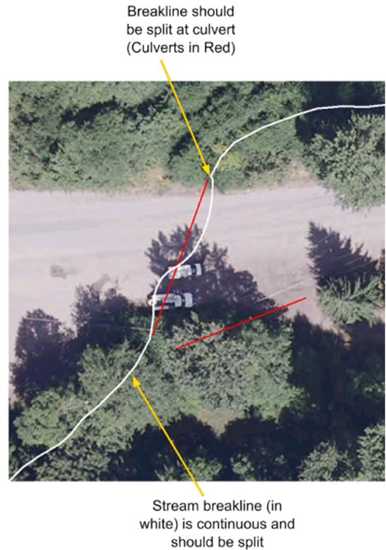
LP360 for ArcGIS® contains a dedicated set of tools for performing and annotating QC problems in LIDAR data sets. The figure below provides an example of an annotated breakline error.
